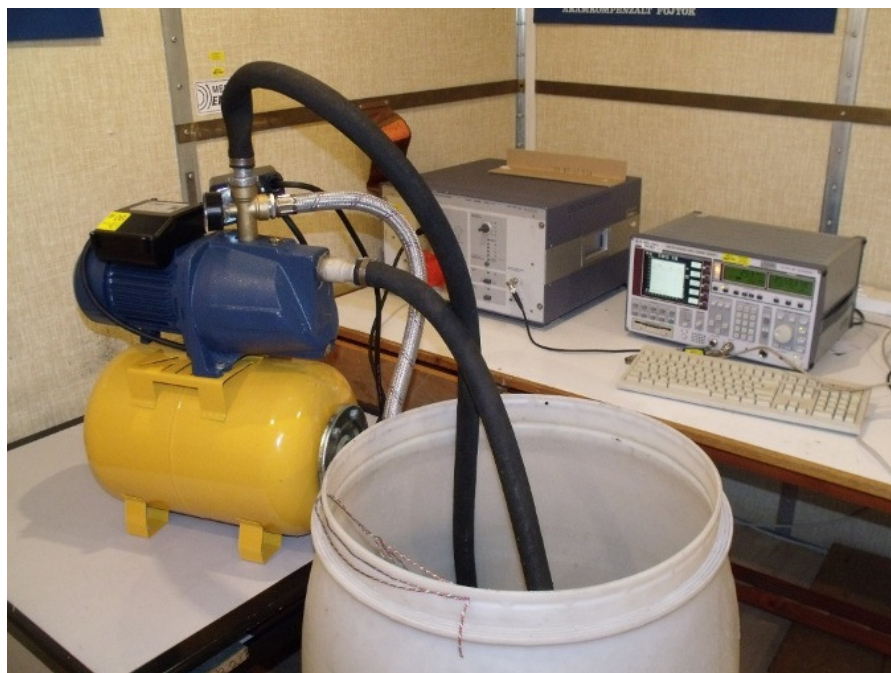
Measurement of disturbance voltage
