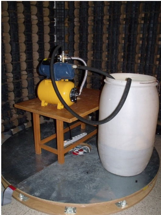
Measurement of radiated disturbances
